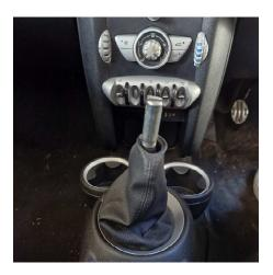
2. Locate and remove the 3 torx 20 bolts 2 in the cup holders and 1 on the rear cup holder.
